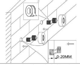
Mount the eccentric feets( cold water side and hot water side).
