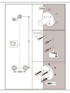
Mark the positions on wall for installing the shower column by referring to dimension drawing.
